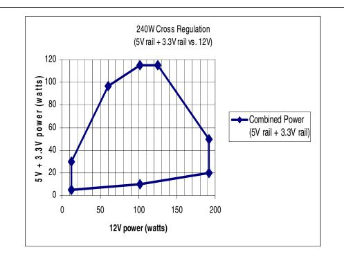
Figure 4. Cross Loading Graph for 240W Configuration
